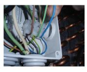
lenoid into the same tree that the main power comes into, but we'll use the terminals on the bottom rather than the ones on the top. Again, like the power cord, the ground (green w/ yellow stripe) goes in the center and the hot leads (blue and brown) go to the left and right. And again the configuration of the hot leads does not matter. Congrats button everything back up and you're ready to go!
