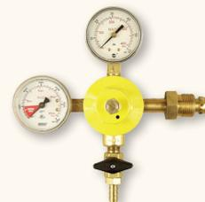
You can adjust the flow of gas by turning the screw in the main body of the regulator. This threaded fitting will usually be screwed all the way out when it is new, but it will not actually come completely apart from the regulator body. To engage it, thread it in slowly till the threads start to connect. The more you thread it in, the more
